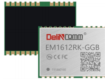
Figure: EM1612RK-GGB Top View
